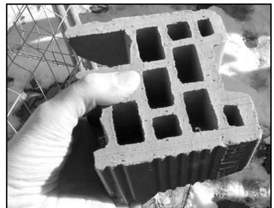
Locally produced building blocks from Marzabotto are energy saving, cheap and require minimum transport
