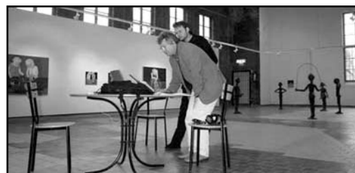
Measuring reverberation time in the Old Boiler House at Kristinehamn
