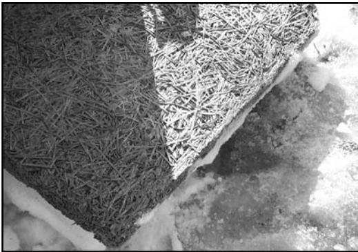
Insulation made of recycled wood or paper is healthy and has low embodied energy
